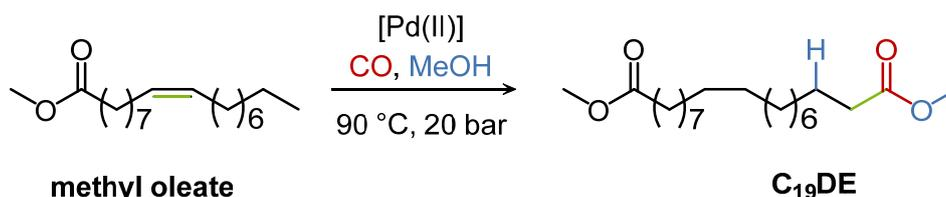
Figure 1 Methoxycarbonylation of methyl oleate to highly linear dimethyl 1,19-nonadecanedioate
